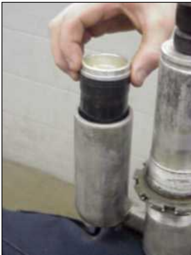
Fig 3 Remove the shock bladder.
