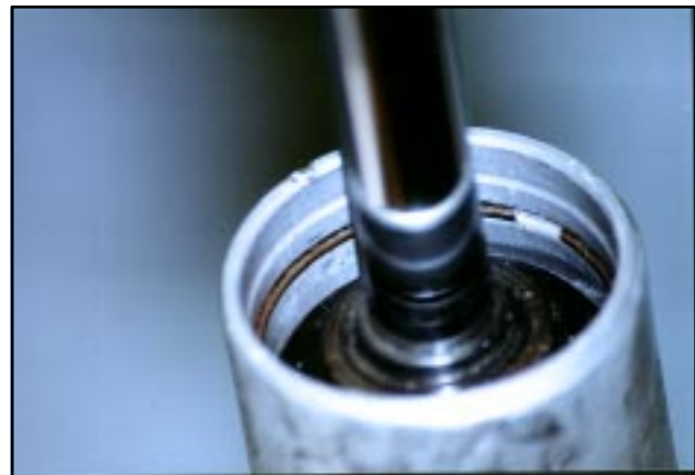
Fig 5 Push down the seal head until the circlip can be removed.
