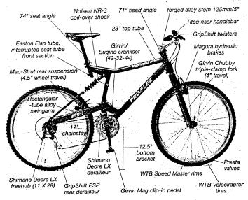
owner decide to try downhill racing later on. To keep the Beast running, grease ports were installed at all pivot locales. No head tube gussetting was used, but we would guess that Easton's butting process included mega-thick sections at the Beast's head-tube junction.
